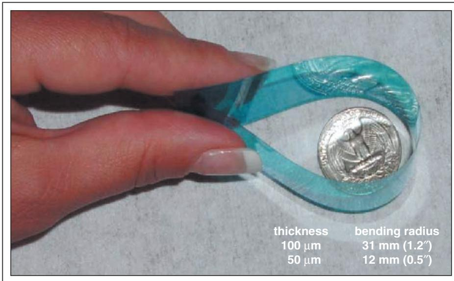
**Fig. 2:** Flexible glass used as armoring in A D Metro's and TouchKO's resistive touch panels. The sample shown is 0.05 mm thick, while the glass used for armoring is 0.1 mm thick. The sample has been dyed blue to make it more visible.
