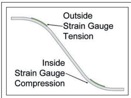
**Fig. 7:** In QSI's InfiniTouch™, the sensors are placed where the beams bend in response to normal forces. The sensors on opposite ends of one beam experience strains with opposite signs in response to normal forces. Lateral forces cause the sensors on a beam to experience the same strain.
