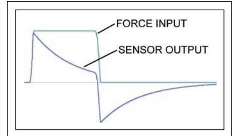
Fig. 4: The typical output of a piezoelectric transducer.
