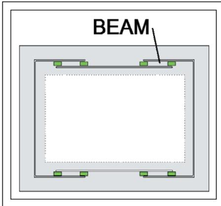
**Fig. 6:** An illustration of the structure of QSI Corp.'s InfiniTouch™ planar touch-panel configuration.
