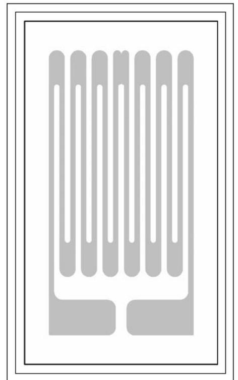
**Fig. 3:** An illustration of a typical strain gauge.
