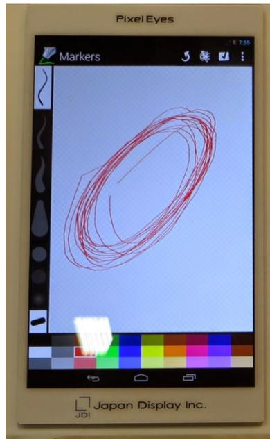
***Japan Display, Inc.’s (JDI’s) latest “Pixel Eyes” hybrid in-cell/on-cell embedded touch is shown here in a 7-inch display with 1,200 x 1,920 pixels, which is 323 ppi. The circles on the screen (drawn as fast as possible with a 1 mm-tip passive stylus) demonstrate quite good performance, with only a couple of lost points. Photo by author.***
