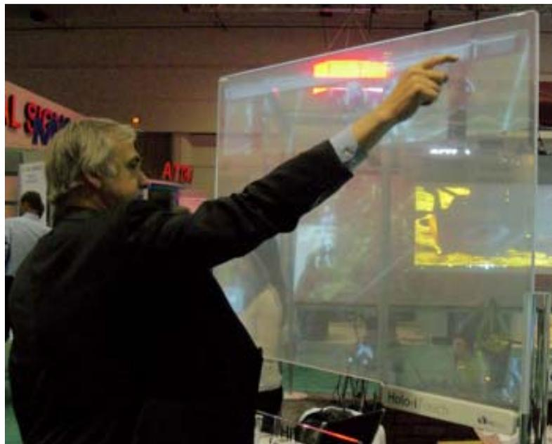
Vislogix's "Holo-iTouch" using Visual Planet's projected-capacitive film
