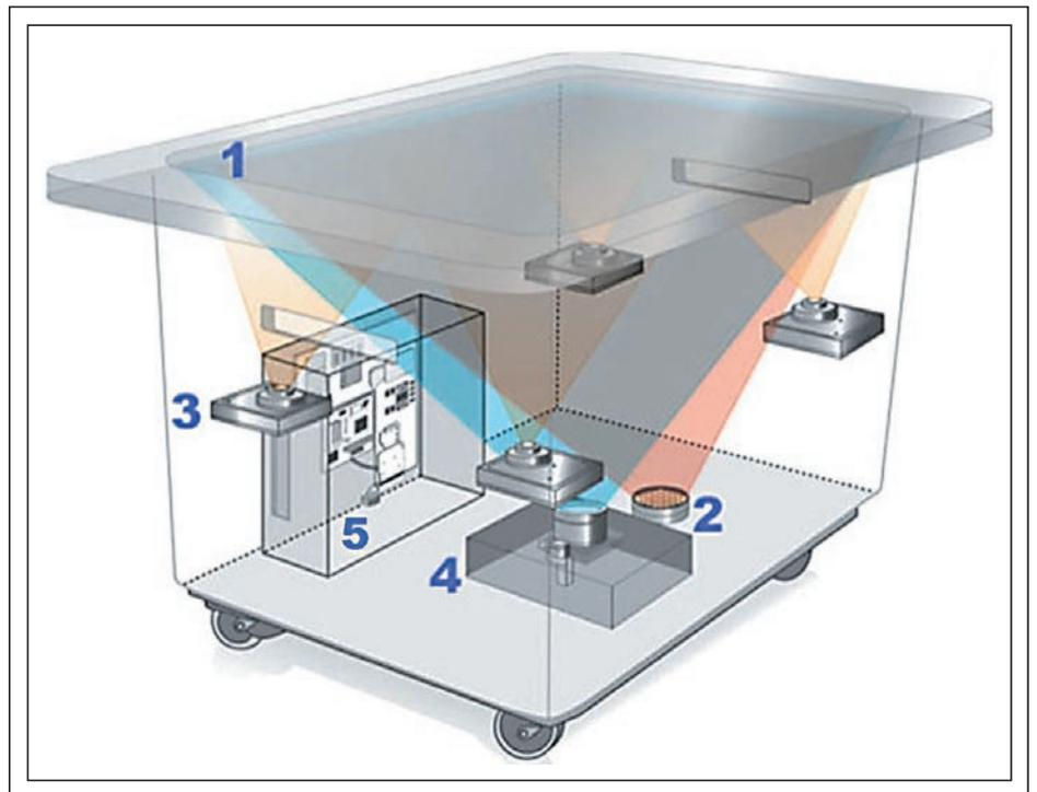
**Fig. 1:** Schematic format of Microsoft's Surface computer product. The components numbered in blue are as follows: (1) acrylic tabletop touch surface with a diffuser; (2) 850-nm infrared light source directed at the underside of the touch surface; (3) infrared camera (one of four with a combined total resolution of 1280 × 960 pixels); (4) Texas Instruments' DLP projector running at 1024 × 768 pixels; (5) desktop computer running a customized version of Microsoft Vista. Source: Microsoft.
