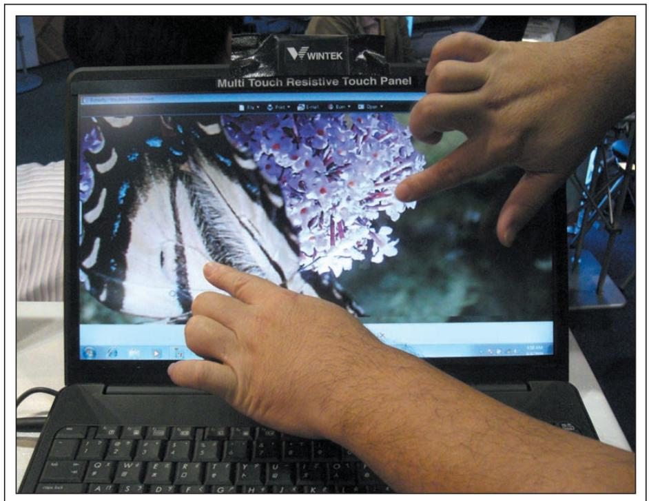
**Fig. 2:** This prototype of a 16-in. wide-aspect digital-resistive multi-touch touch screen from Wintek is installed in a laptop. This is probably the largest digital-resistive touch screen that has been shown to date.
