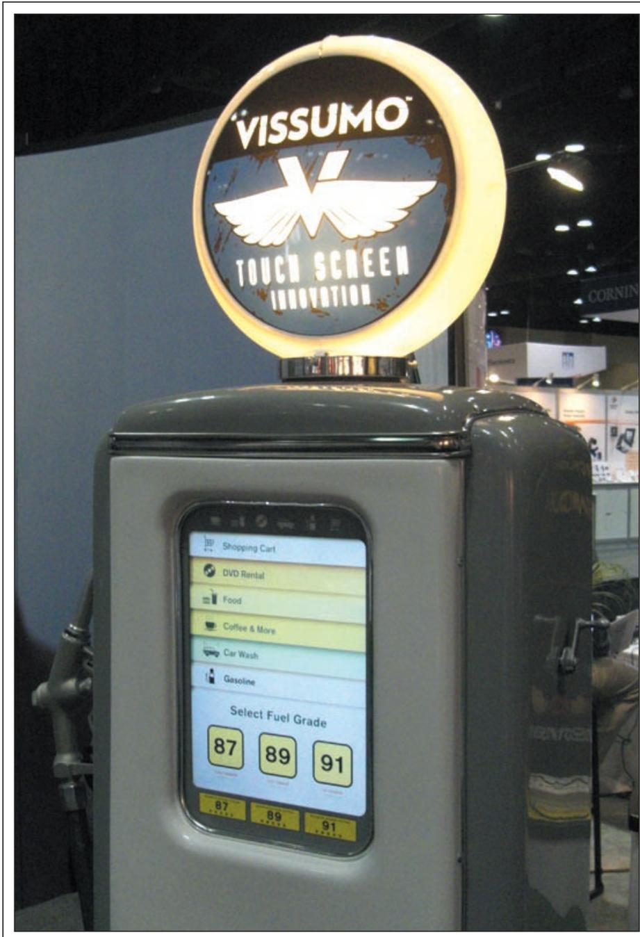
**Fig. 3:** This display features a mockup of a gas pump using Vissumo’s force-sensing touch screen. Rugged outdoor touch applications such as this take advantage of force-sensing’s high degree of resistance to adverse environmental conditions.
