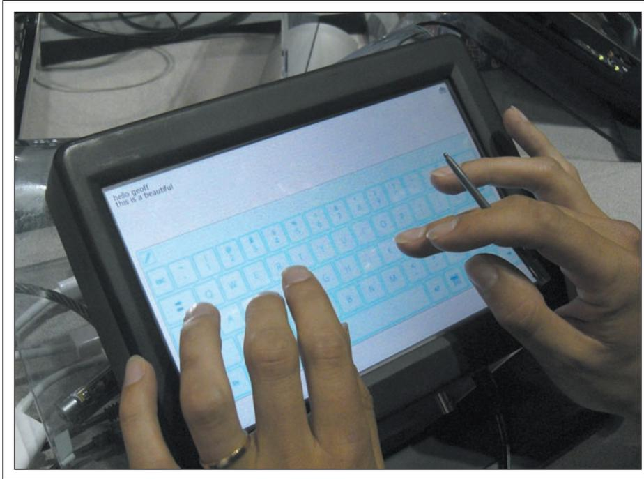
**Fig. 1:** This on-screen keyboard used a digital-resistive touch screen from Stantum. The booth staff-person was able to touch type on this screen even without tactile feedback.
