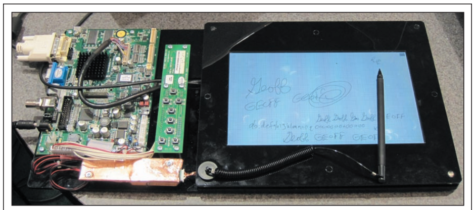
Fig. 2: Above is Stantum’s very-high-resolution (0.65 mm) analog multi-touch resistive (AMR) touch screen, showing extremely fine digital ink. The touch screen uses four Sitronix controller chips around the edge (under the bezel). The left side of the photo is a standard video card used to drive the display electronics on the right.
