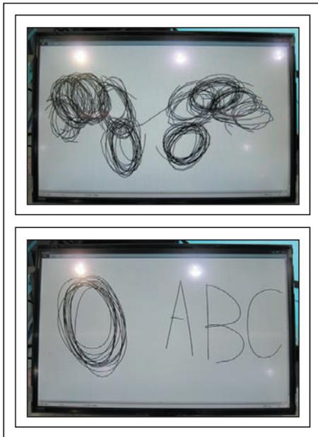
**Fig. 2:** Top: Wacom's 22-in. pro-cap touch screen shows a worst-case test with 10 fingers drawing circles as fast as possible. Bottom: An average-case test uses two fingers, one drawing circles at a moderate pace while the other writes the letters A-B-C. Photo courtesy Geoff Walker.
