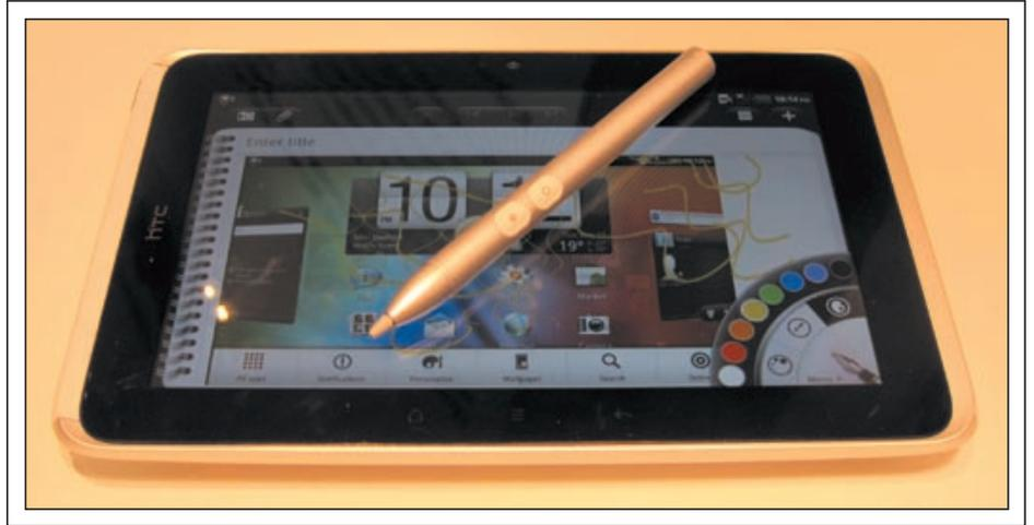
**Fig. 3:** The HTC Flyer Android tablet with a 7-in. display and N-trig's dual-mode (pen and finger) pro-cap touch screen. With the product thickness at only 0.5 in., there is no internal storage for the stylus. Photo courtesy Geoff Walker.
