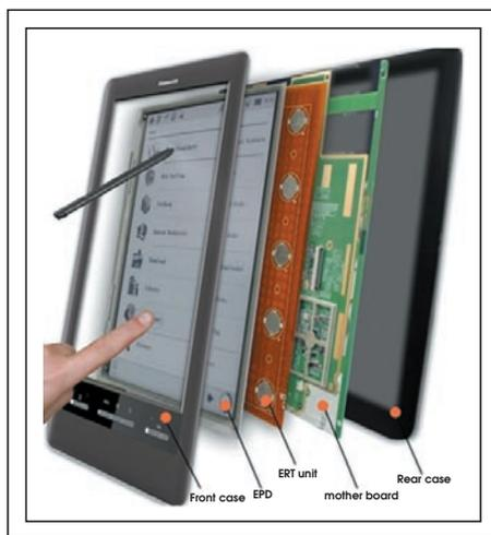
**Fig. 5:** In Hanvon's dual-mode (pen and finger) EMR digitizer, the sensor board (labeled "ERT unit") is shown inserted between the electronic-paper display (EPD) and the motherboard in an e-Reader. The circles shown on the sensor board represent one column of an array of force-sensing piezo capacitors. Image source: Hanvon.
