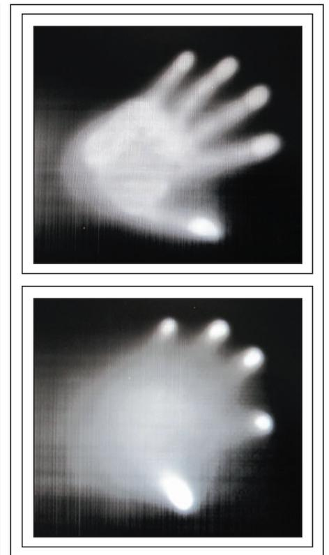
**Fig. 4:** These photographs show the sensor-array output (displayed on a secondary LCD) from Samsung's 40-in. in-cell optical ("PixelSense") LCD. Top: The author's palm flat against the display. Bottom: Fingertips only. Photo courtesy Geoff Walker.
