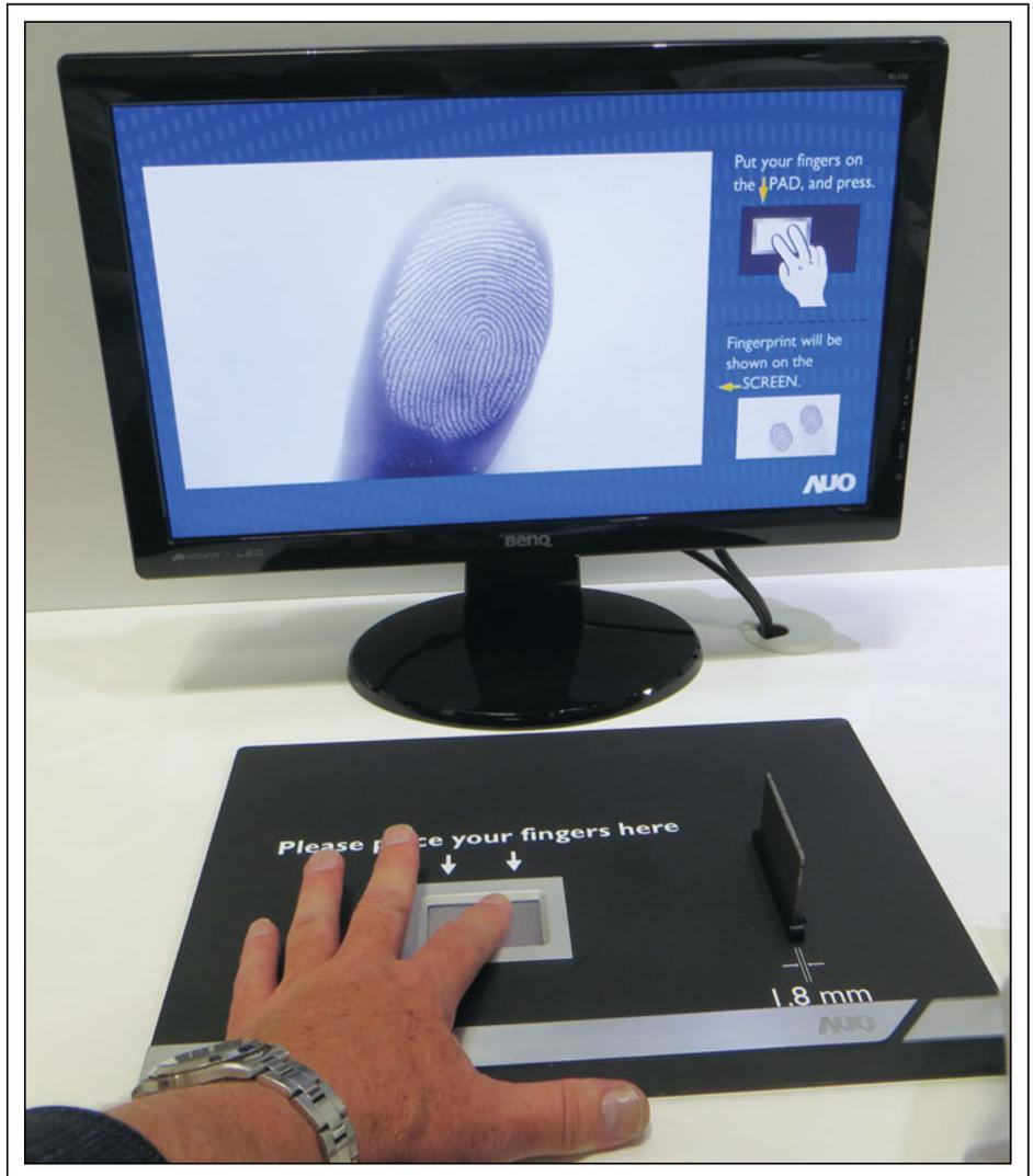
*Fig. 2: AUO's 508-ppi fingerprint sensor shows the author's left index fingerprint. The sensor is basically a display backplane without pixel drive electronics, so the entire pixel can be used for optical sensing. Photo courtesy Geoff Walker.*
